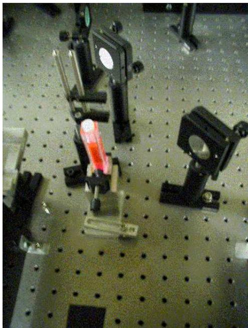
Figure C.5: Dye laser 2 amplifier.
