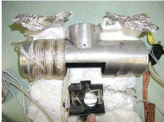
Figure 3.7: Oven with Cs cell inside.
