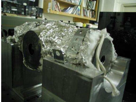
Figure 3.8: View of the side and end windows of the oven.
